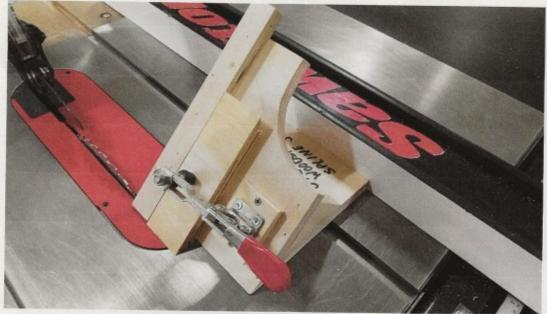
In order to safely cut this groove in your miter joint, use the jig in the photo below.
