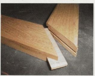
Therefore, the miter joint must be reinforced somehow and we do this with a spline. A spline is a piece of wood or a biscuit that is glued into a recess made in the joint.
