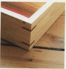
The third orientation of a spline in a miter joint is shown in the photo below. This type of spline is typically decorative and can be made to show off the spline as well as the beauty of the box.
